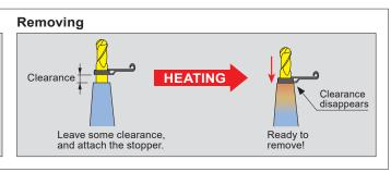
Simply adjustment for cutting tool projection and insertion length.
