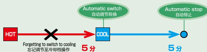
Even if you forget to switch to cooling operation, this unit automatically switches to the cooling operation 5 minutes after the heating operation started to prevent overheating problems.
